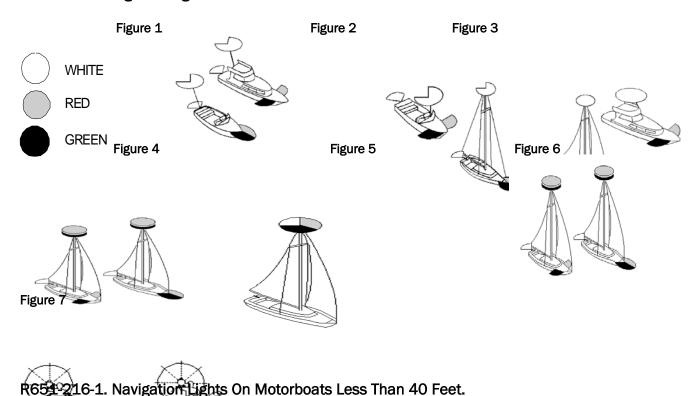
Motorboats of less than 40 feet in length shall exhibit the navigation lights shown in either figure 1, 2, or 3.
